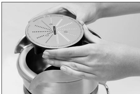
4. Place the puree insert into the filter bowl surround, making sure the warning label on the handle is facing upwards.
